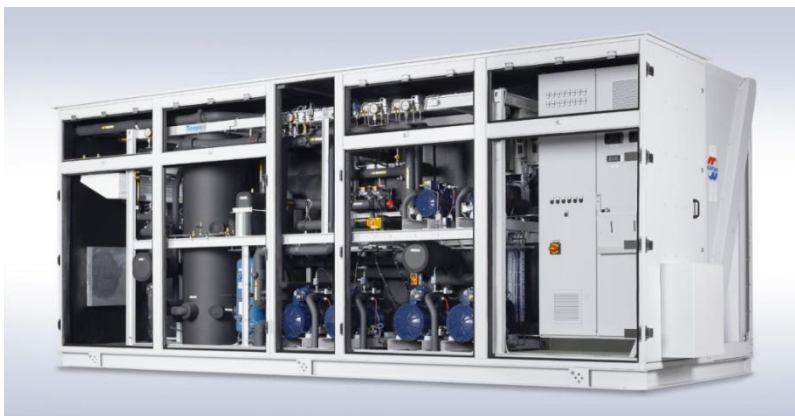
Figure 5 CO2 booster package system, with semi-hermetic reciprocating compressor, oil separator, control cabinet, etc. for supermarket refrigeration
