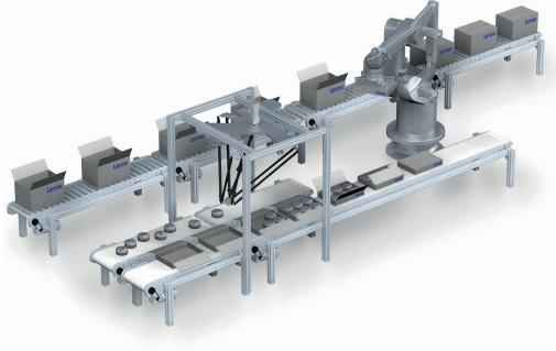
FAST goes robotics: Ready-made robotics modules make it extremely easy to integrate kinematics into the entire automation process. Technology modules for Pick & Place applications are available for this purpose, with models designed for different kinds of kinematics. A fully functional robotics core is already integrated to ensure the greatest possible degree of freedom.
